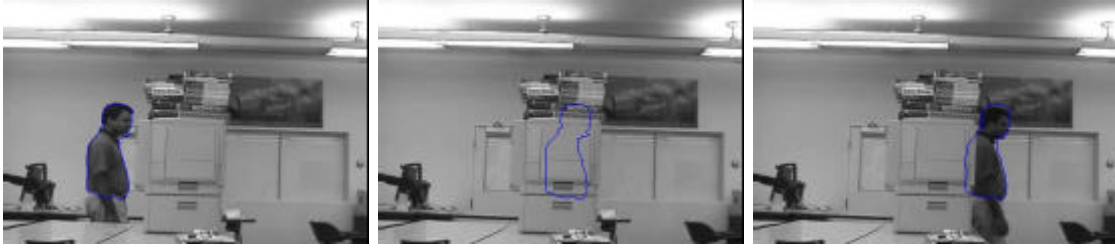
Figure 1.6: The Georgia Tech active contours algorithm has the ability to track a target even when it moves through an occlusion.
