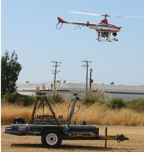
Figure 1.4: The Berkeley Aerobot is an R-50 UAV that uses a designated target to estimate its position.
